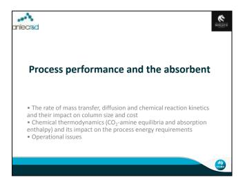
The way a capture process performs is controlled by the complex interplay between a number of factors. There is: the rate at which  $CO_2$  is absorbed and the amount that can be absorbed; the energy that must be input to heat the solvent and release  $CO_2$ ; degradation of the solvent via oxidation, heating and reactions with  $SO_x$  and  $NO_x$ ; corrosion of the plant; and many more.
