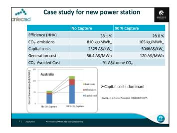
This slide gives relevant data for the power plant efficiency,  $CO_2$  emissions, capital costs, generation cost and  $CO_2$ -avoided cost for a new power station, in the situation without capture and with 90%  $CO_2$  capture. Although the emissions are significantly reduce the increase in the capital cost and electricity generation cost is significant.
