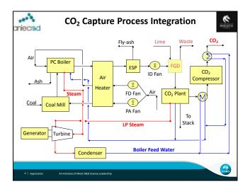
The figure shows how a capture plant could be integrated into a power station. In this case the flue gas pre-treatment would consist of an electro-static precipitator (ESP) and flue gas desulphurisation (FGD) in addition to flue gas cooling. Low pressure (LP) steam is used to regenerate the solvent and the condensate is returned to the pulverised coal (PC) fired boiler. This steam is then not available to generate electricity.
